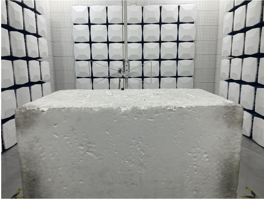
Radiated Emission Test Setup 1 30 MHz - 1 GHz (Transmitter tests)
